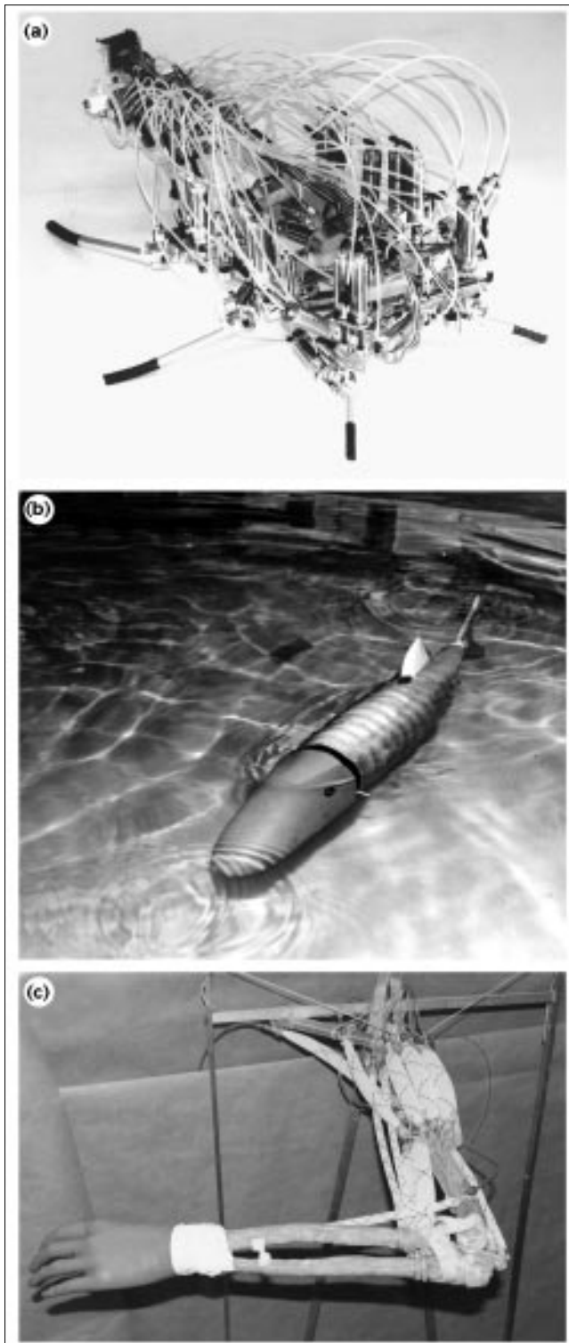
Several recent examples of biorobots. (a) A cockroach-like hexapod robot based on the leg kinematics of Blaberus discoidalis [24**]. (b) A robotic fish inspired by the chain pickerel Esox niger [29**]. Photograph courtesy of John Muir Kumph. (c) A biorobotic model of the human arm [46]. Photograph courtesy of Blake Hannaford.
